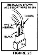
5 - Insert the three-pin (P69) plug from the control box
